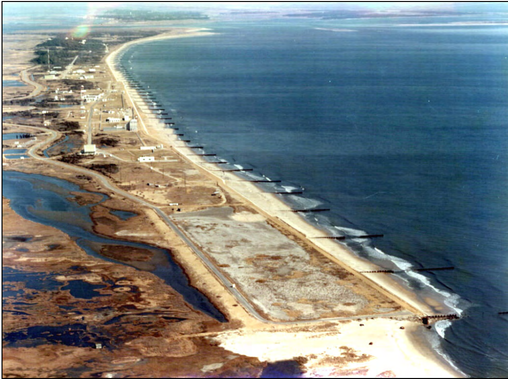
Figure 8. By 1976, shoreline had moved to approximately halfway mark on groins. Chincoteague Inlet and Fishing Point can be seen in upper part of frame. NASA photograph 76-142, courtesy of Goddard Space Flight Center.
