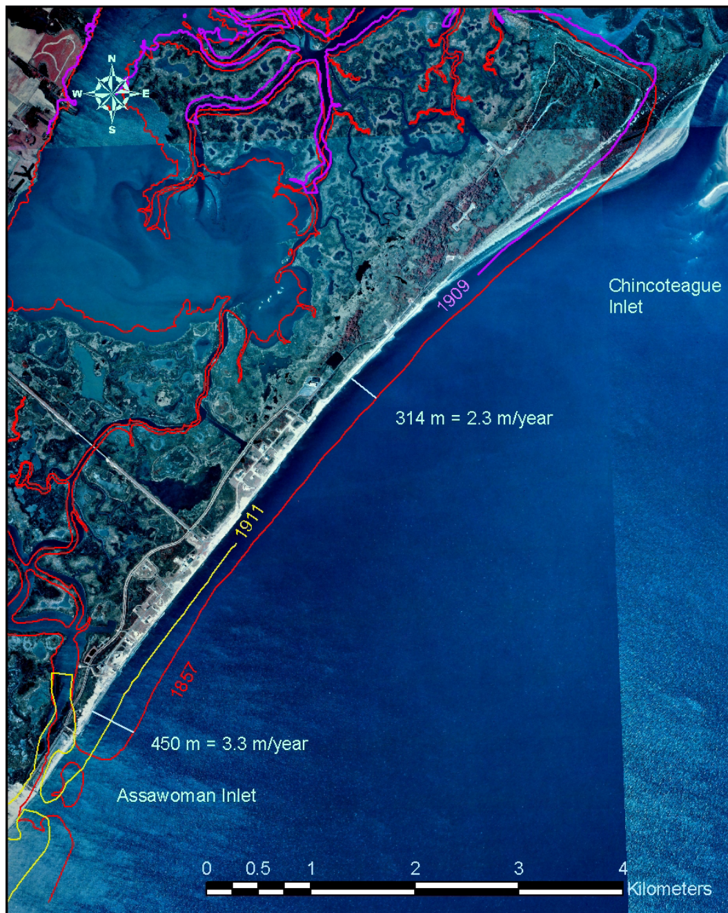
Figure 4. Shoreline changes at Wallops Island from 1857 to mid-1980s. Shoreline data from NOAA and state of Virginia. NASA's facilities are located on narrow sand strip. Aerial photograph: 1994 Digital Ortho Quarter Quadrangle downloaded from Virginia Economic Development Partnership.
