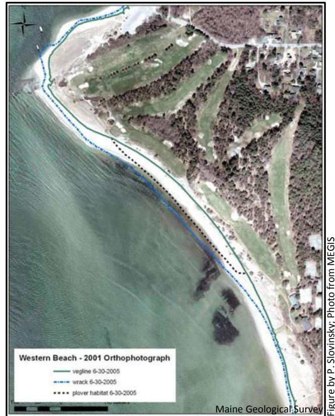
Figure 18. 2001 aerial orthophotograph with the field surveyed location of the vegetation line, wrack line, and fenced shorebird nesting area from June 2005.
