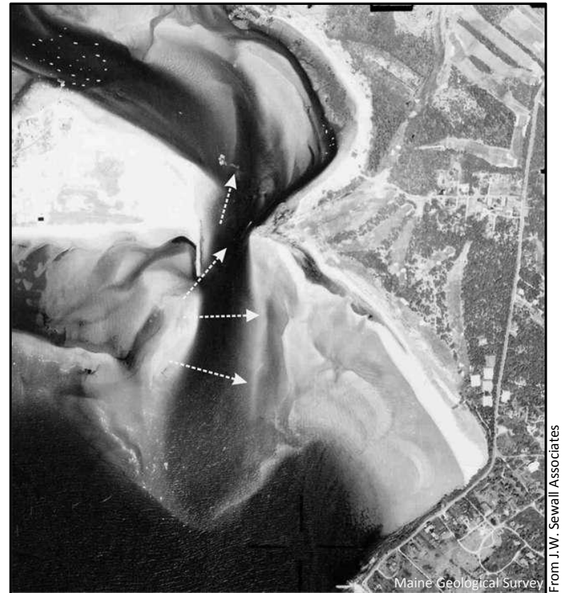
Figure 3. Aerial image from 1962 showing the morphology of the Scarborough River ebb tidal shoals and the newly built jetty. White arrows show the direction of shoal bypassing prior to the 1962 stabilization.
