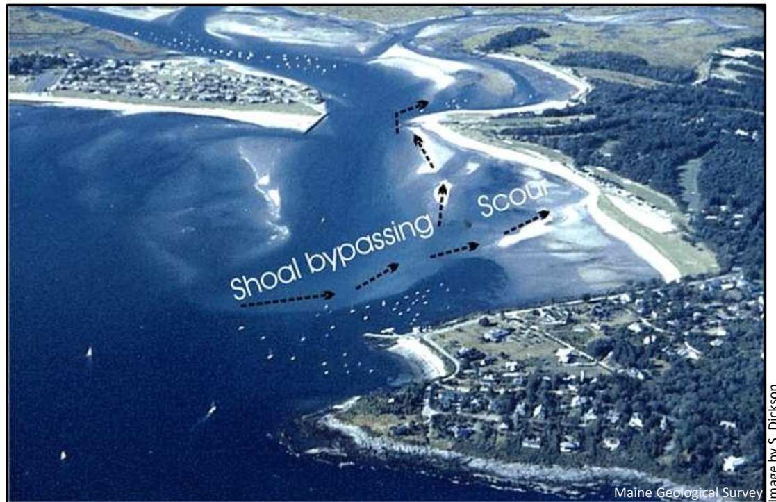
Figure 5. Oblique aerial photograph from 1987 showing shoal bypassing occurring, but farther offshore. The jetty causes the buildup of a sand bar that acts as a littoral barrier, and shoals must come around this barrier in order to migrate to Western Beach. Note the shoal locations off of Western Beach.
