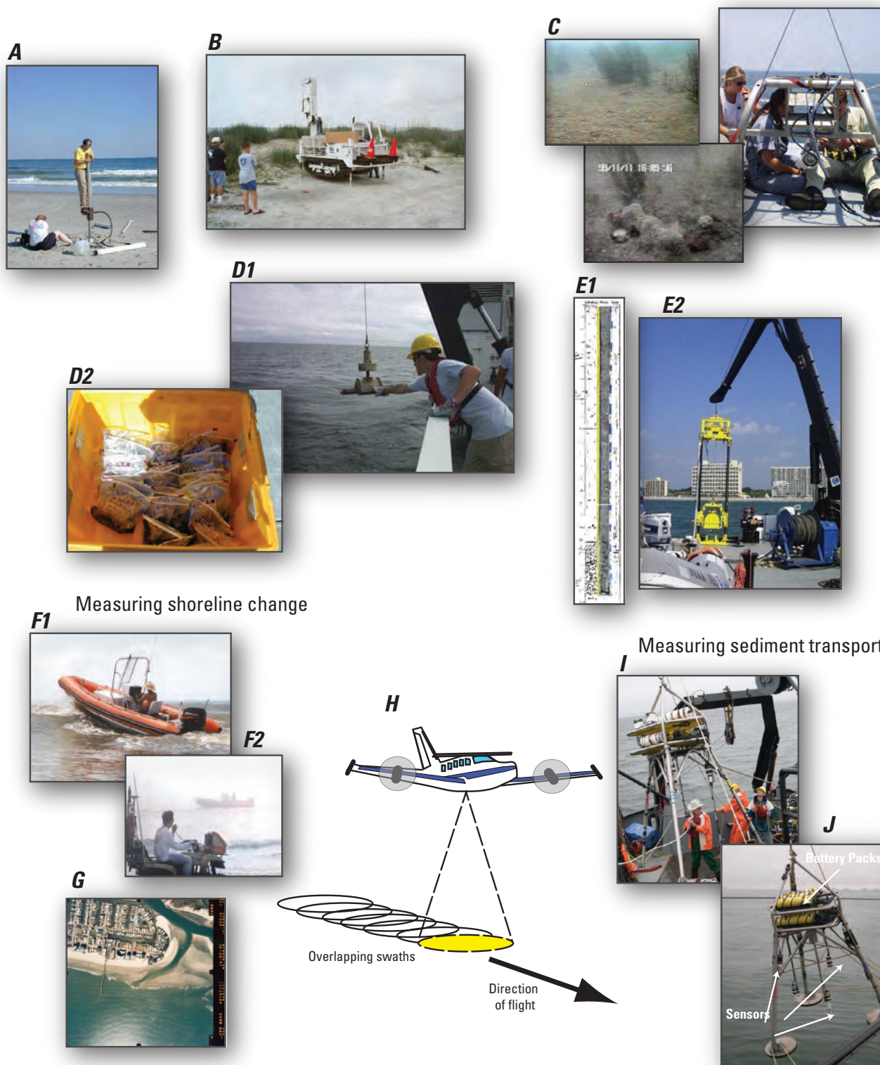
Figure 2.2B. Mapping operations of the SCCES include (A) collection of sediment core on the beach, (B) large coring rig for deep sampling, (C) video camera used to collect images of the seafloor, (D1) grab sampler used to collect sediment from the seafloor, (D2) sediment samples stored in bags for laboratory analysis, (E1) photograph of a sediment core, (E2) collection of offshore sediment with Vibracores, (F1) rigid-hull inflatable boat measuring beach profiles in nearshore area, (F2) ATV measuring beach profiles onshore, (G) aerial photograph used in shoreline-change analysis of North Myrtle Beach, (H) LIDAR systems rapidly map topography over extensive areas of coast, and (I) and (J) deployment of oceanographic instruments on a tripod (rigid three-leg structure) that will be anchored to the seafloor.
