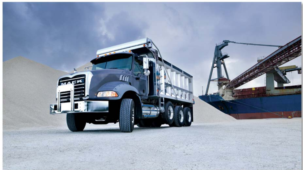
Figure 5.1: Typical four-axel road truck used to haul sand from the sand mine to the project site.
