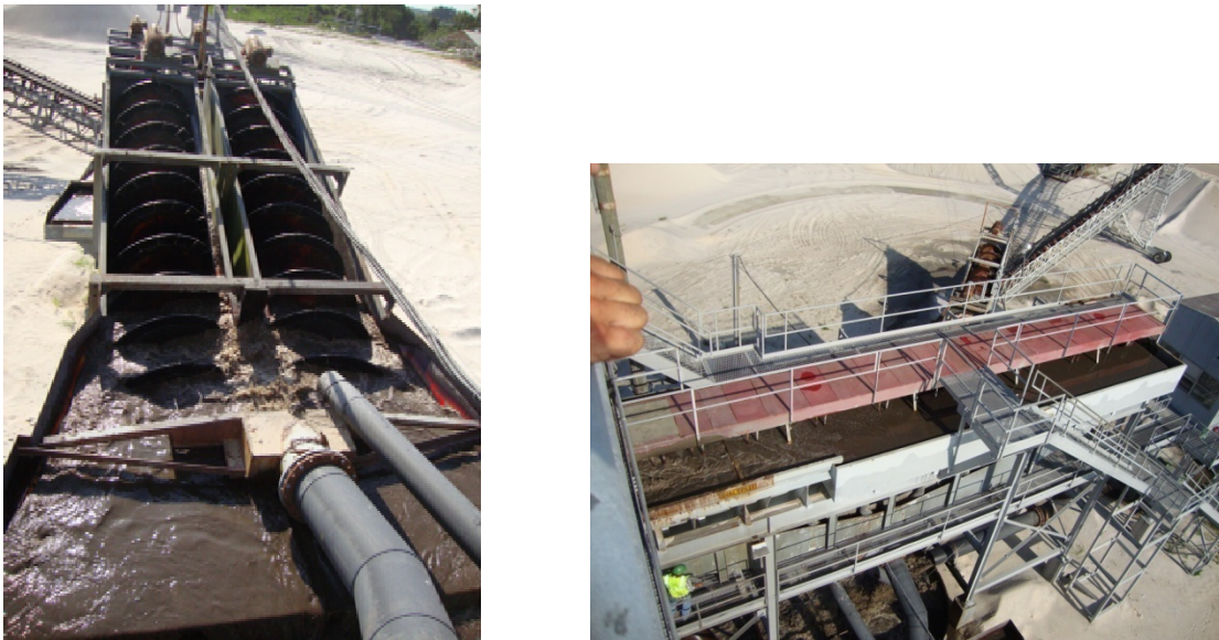
Figure A.4: Jahna Ortona dewatering screws (left) and processing plant (right).
