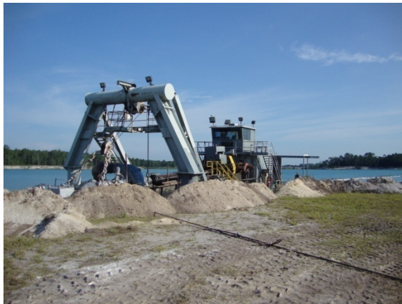
Figure A.9: Jahna Greenbay cutter head dredge (left) and processing plant (right).
