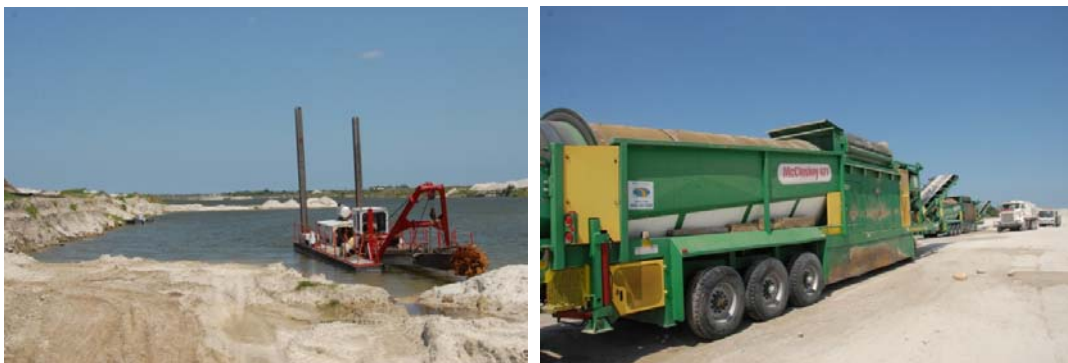
Figure A.17: Fischer Ranch Road Lake mine with a cutter-head (left) and Trommel (right).
