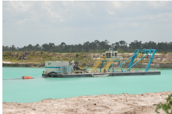
Figure A.2: Stewart Immokalee hydraulic dredge (left) and processing plant (right).
