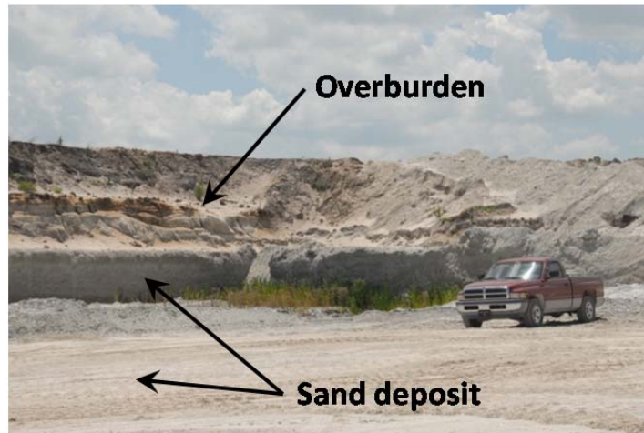
Figure A.16: The Stewart Ft. Pierce mine showing thick layers of overburden and limestone which were removed to expose the top of the sand deposit.
