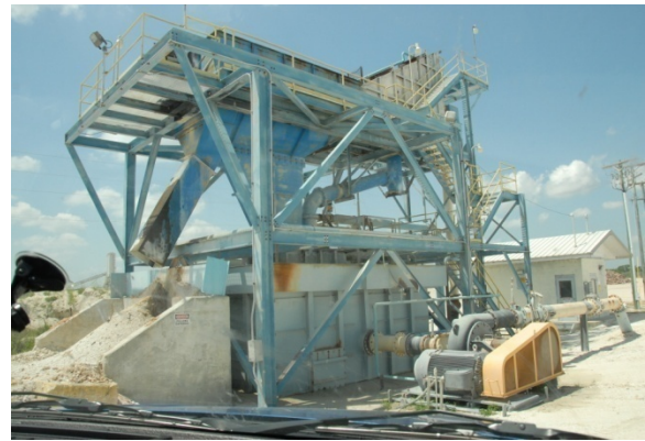
Figure A.12: Initial processing removing large material (left) and the hydraulic dredge (right) at Cemex Lake Wales.
