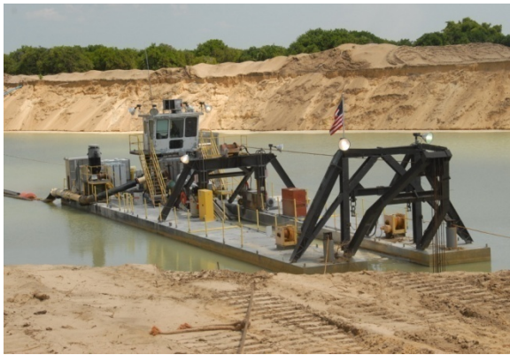
Figure A.12: Initial processing removing large material (left) and the hydraulic dredge (right) at Cemex Lake Wales.
