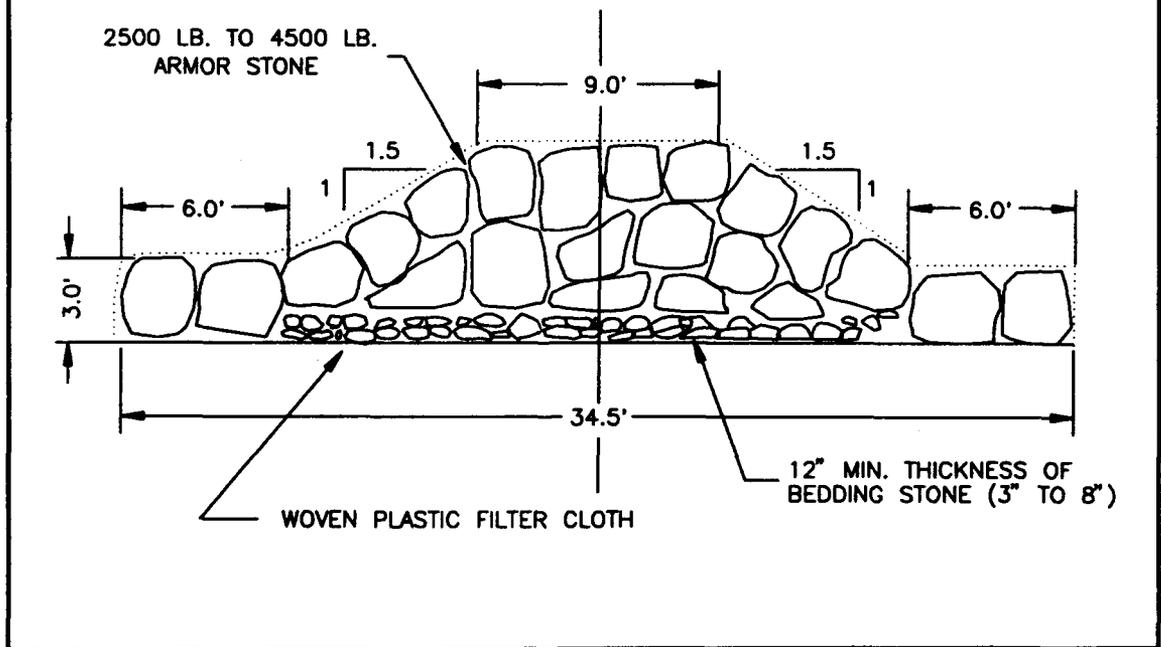
Figure 48. Example of a low-crested breakwater at Anne Arundel County, Maryland (Fulford and Usab 1992)
