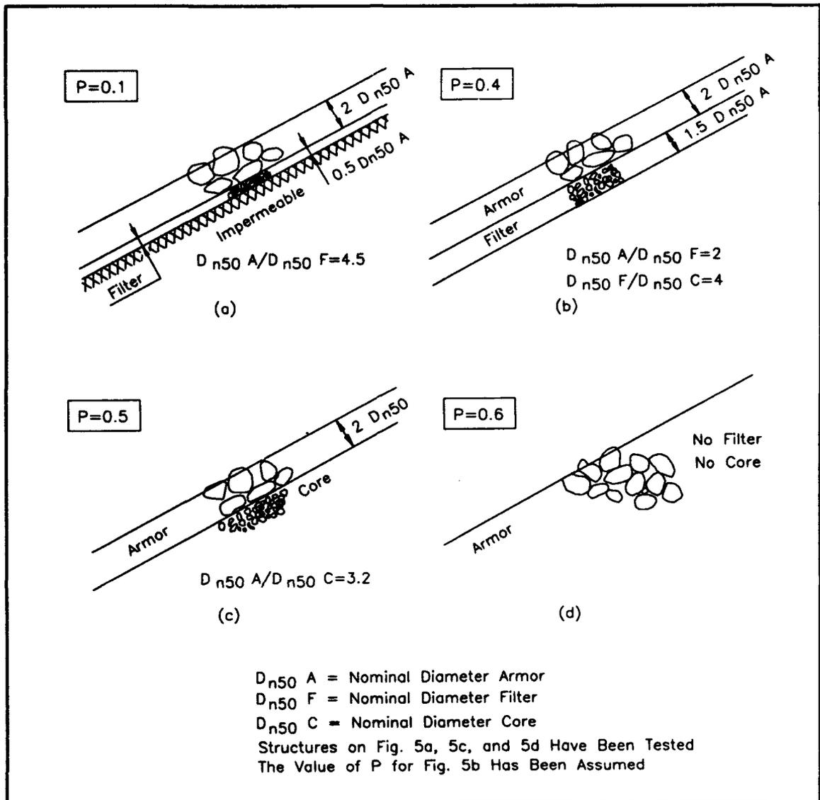
Figure 47. Permeability coefficient  $P$  (Van der Meer 1987)
