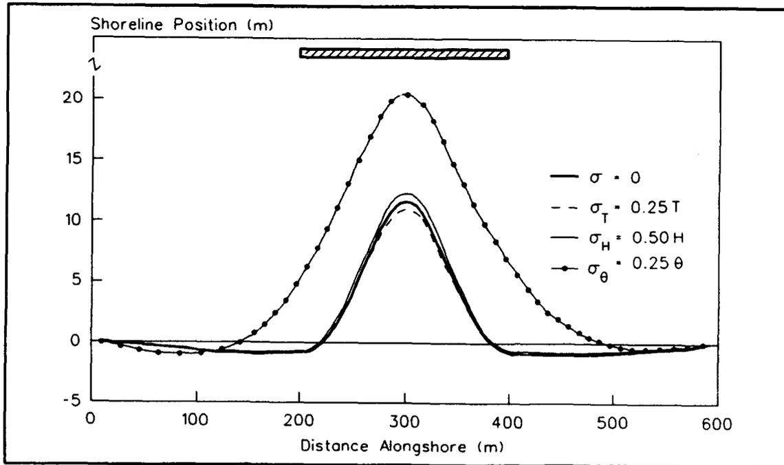
Figure 32. Influence of wave variability on shoreline change behind a detached breakwater (Hanson and Kraus 1990)
