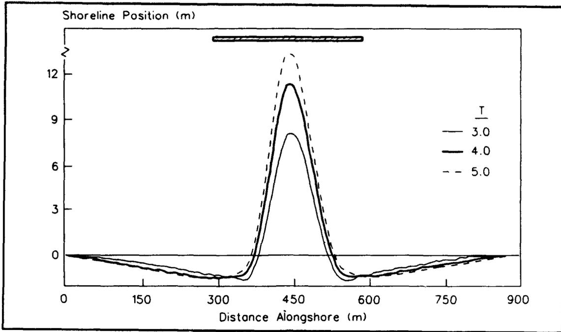
Figure 31. Influence of varying wave period on shoreline change behind a detached breakwater (Hanson and Kraus 1990)
