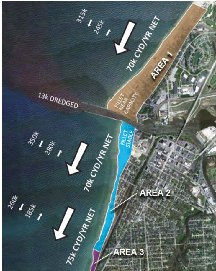
Figure 20: Graphic representation of longshore sediment transport
