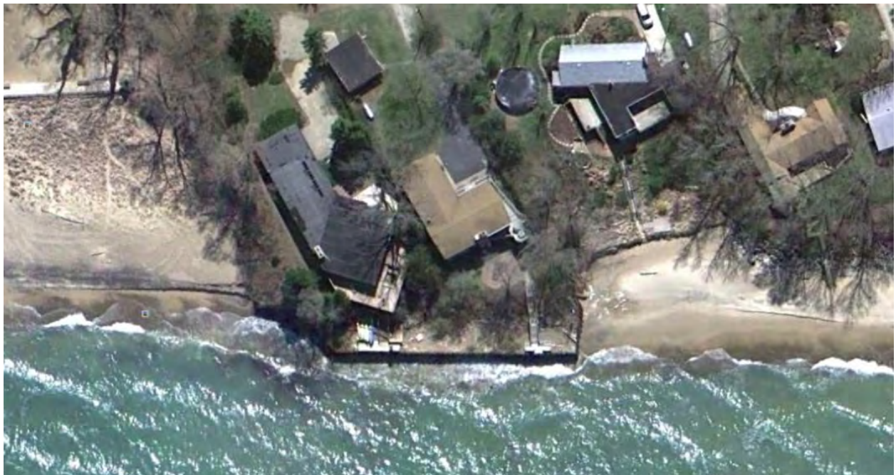
Figure 31: Example of flanking in southern Berrien County. Note how this failure has resulted in the loss of the public trust property lakeward of the NOHWM and public passage is only possible in the lake itself.
