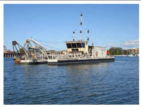
Figure 5-1 400mm Cutter Suction Dredge (Photo Courtesy of Hall Contracting Pty Ltd)
