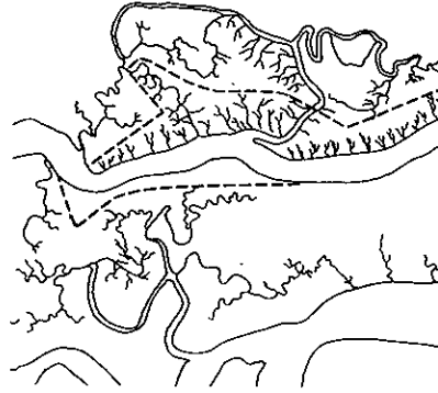
Fig. 4. Black and white aerial photograph (a) documenting the present course of a major stream channel in coastal Georgia along with a visual interpretation (b) of the same area, defining the former stream channel by a dotted line.
