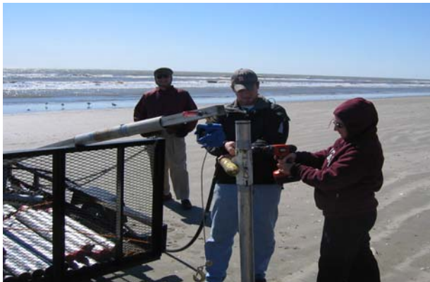
Installing vibra-core head
