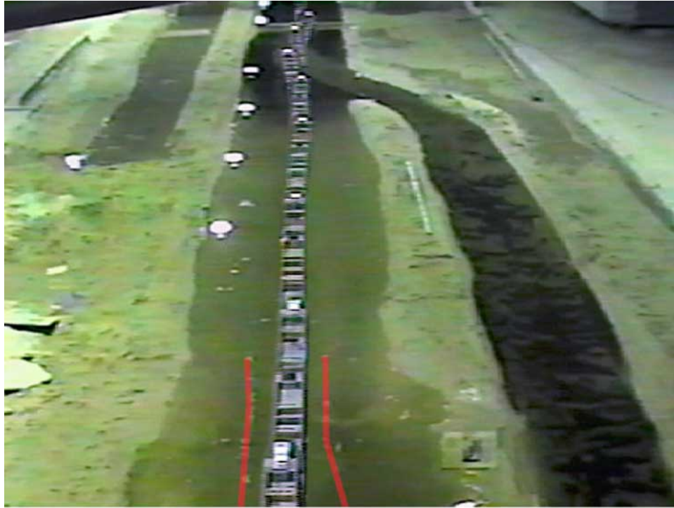
Figure 25. Flow west to east with bridge three tow lengths from confluence, tow moving east to west
