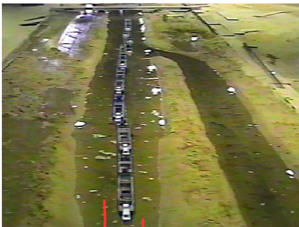
Figure 22. Flow east to west with bridge three tow lengths from confluence, tow moving west to east
