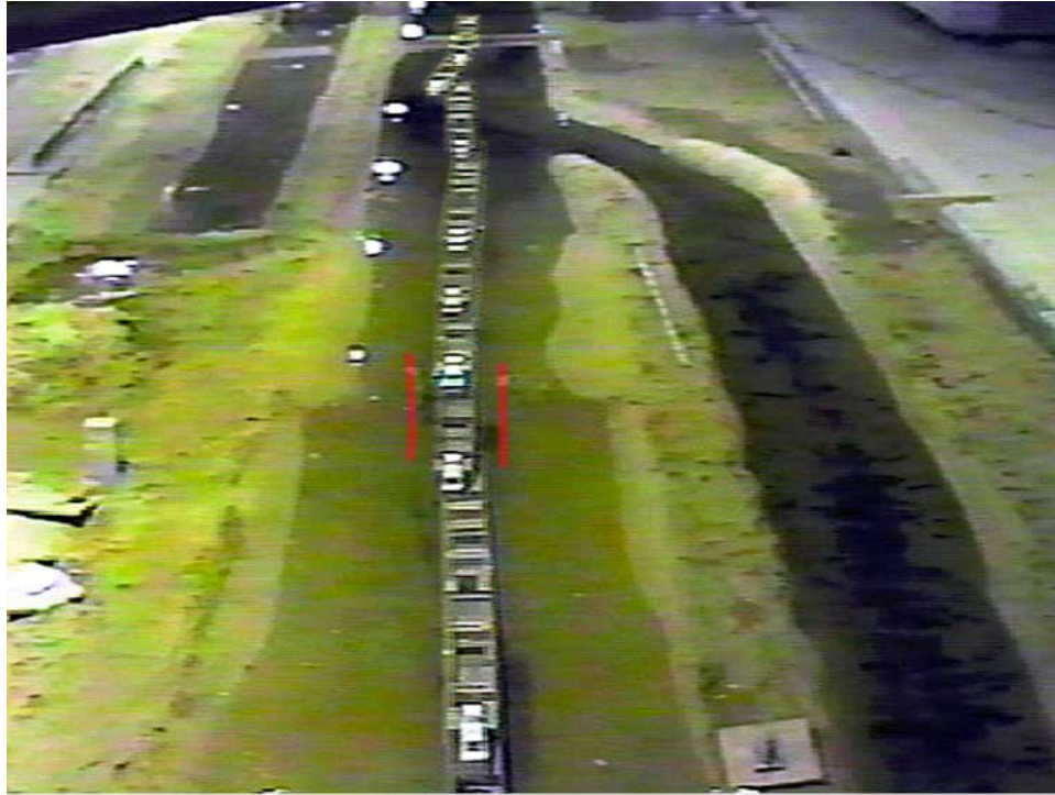
Figure 29. Flow east to west with bridge two tow lengths from confluence, tow moving west to east
