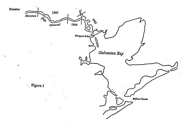
The channel is at present 40 feet deep and 400 feet wide. It was dredged out of portions of Buffalo Bayou and the San Jacinto River in 1914. The original channel was 25 feet deep. In 1925 the channel was deepened to 30 feet and brought to its present depth in 1966. The waterway receives fresh water from approximately 400 industrial and municipal wastewater dischargers, 13 tributaries, and the San Jacinto River.
