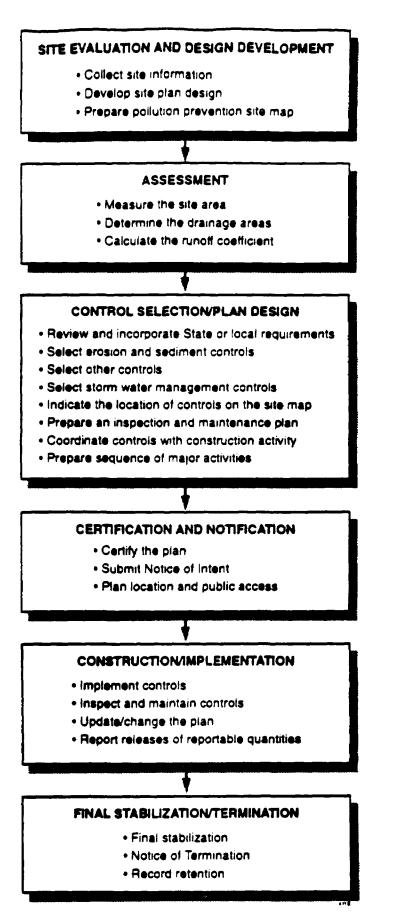
SIX PHASES FOR DEVELOPING AND IMPLEMENTING CONSTRUCTION STORM WATER POLLUTION PREVENTION PLANS
