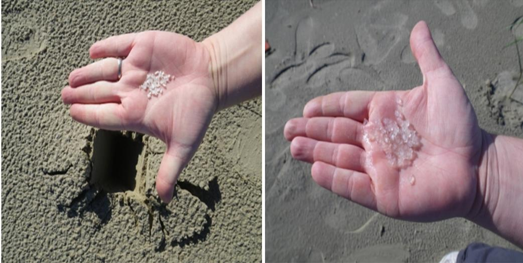
**Figure 8. Soil Moist dry (left) and wet (right)**
