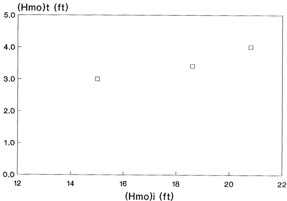
Figure 20. Wave transmission through breakwater, Plan 3
