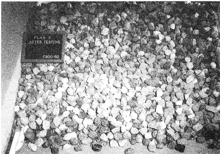
Photo 32. Plan 5, after 24-ft waves, sea-side view
