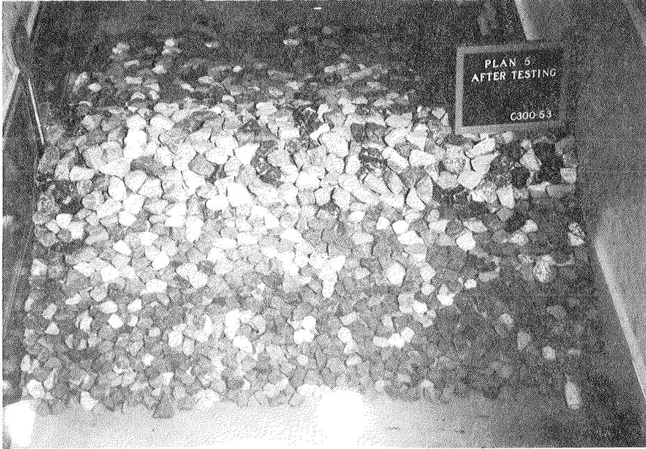
Photo 27. Plan 5, after 16-ft waves, harbor-side view
