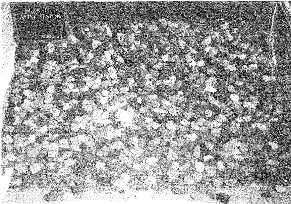
Photo 29. Plan 5, after 20-ft waves, sea-side view
