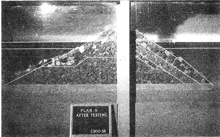
Photo 31. Plan 5, after 24-ft waves, side view
