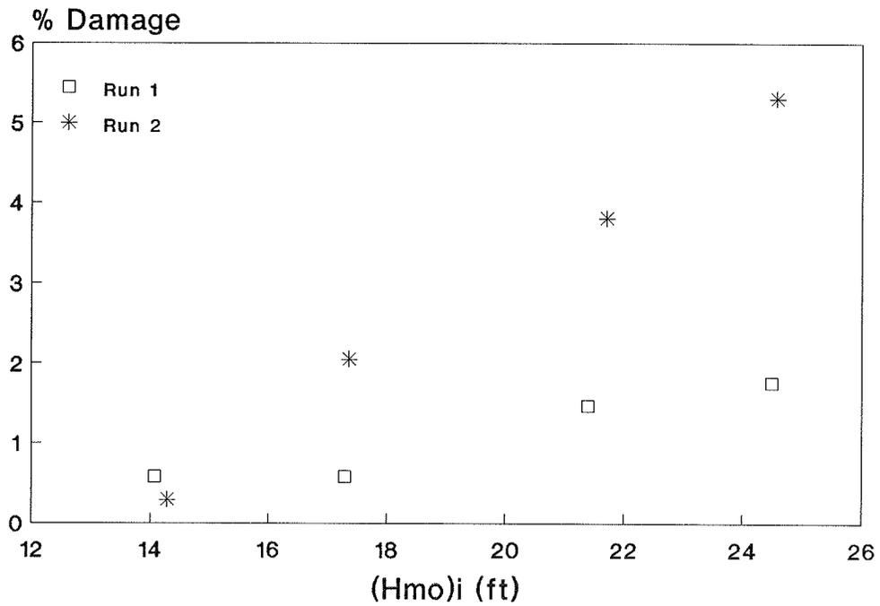
Figure 25. Harbor-side damage, Plan 5, "A-1" Stone
