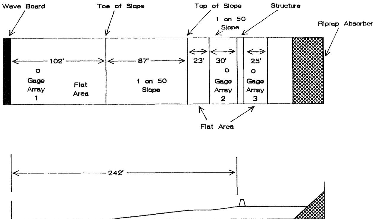
Figure 3. Wave tank used in study
