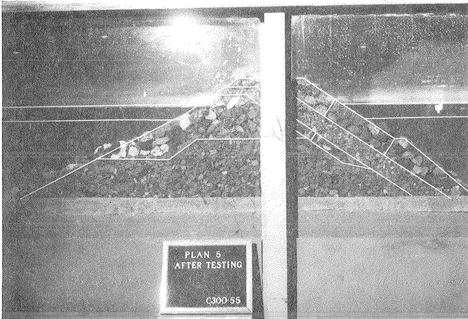
Photo 28. Plan 5, after 20-ft waves, side view
