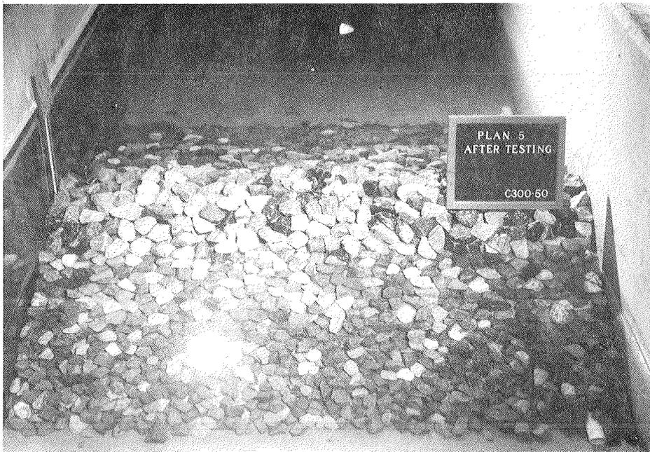
Photo 24. Plan 5, after 13-ft waves, harbor-side view
