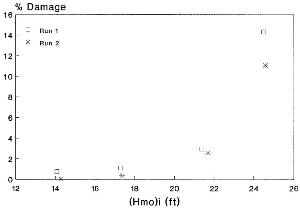
Figure 24. Harbor-side damage, Plan 5, "A" Stone
