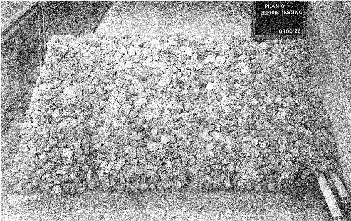
Photo 15. Plan 3, before testing, harbor-side view
