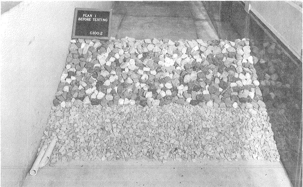
Photo 2. Plan 1, before testing, sea-side view
