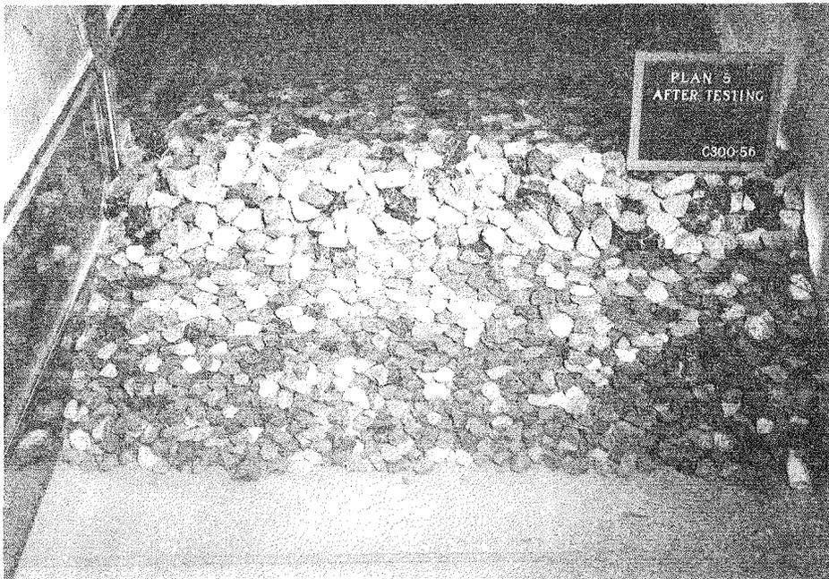
Photo 30. Plan 5, after 20-ft waves, harbor-side view
