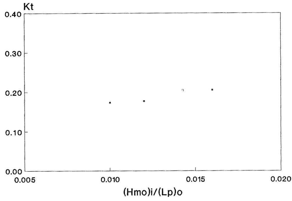
Figure A4. Nondimensional wave transmission, Plan 4
