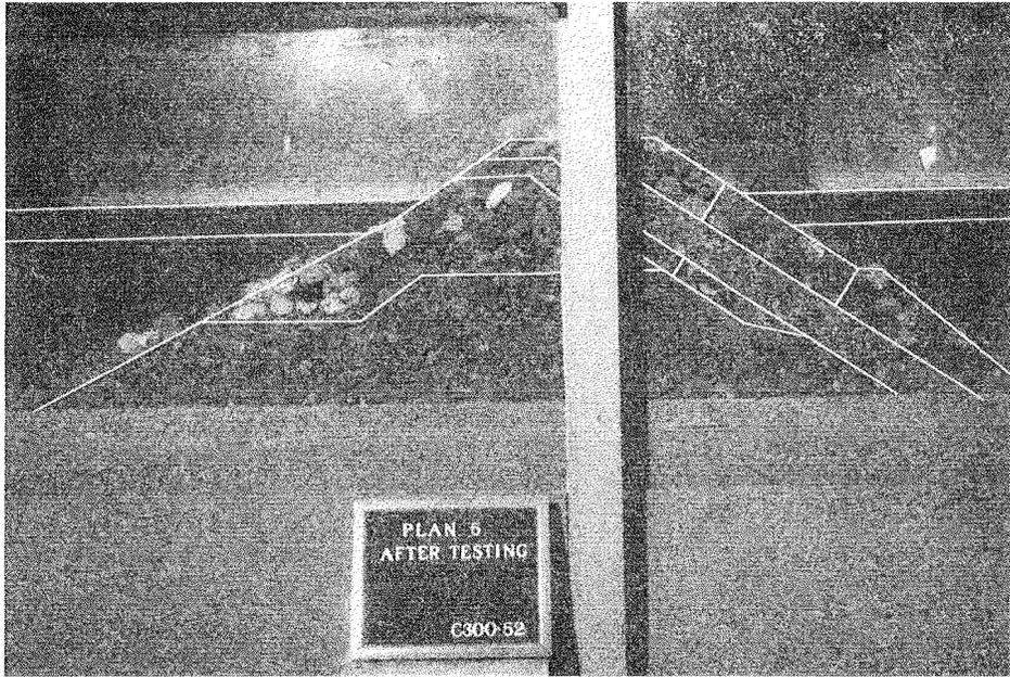
Photo 25. Plan 5, after 16-ft waves, side view
