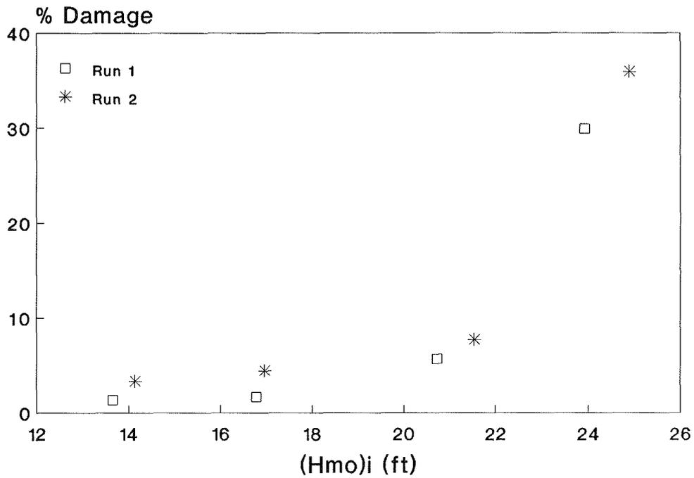
Figure 10. Harbor-side damage, Plan 2, "A" Stone
