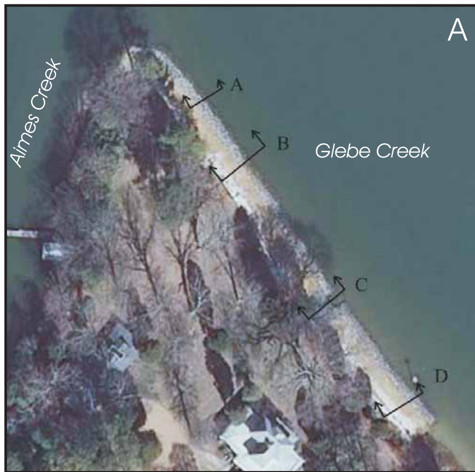
Figure 4-8. Longwood University's Hull Springs Farm on Glebe Creek. A) Before the shoreline project, the bank is eroding in front of the Manor House. B) After the project, the shore zone was widened with sand behind the sills.
