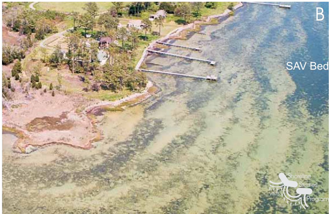
Figure 2-4. Photos showing nearshore bars and submerged aquatic vegetation. A) A VGIN 2009 photo shows the channel into Cranes Creek in Northumberland County, Virginia. Sand bars north of the channel will attenuate waves while the shoreline adjacent to the channel has no bars and will feel the full effect of the waves impacting the shoreline. B) A VIMS aerial photo of Pond Point on the East River in Mathews, Virginia (dated 21 April 2009) showing extensive SAV in the nearshore, as well as sand bars.
