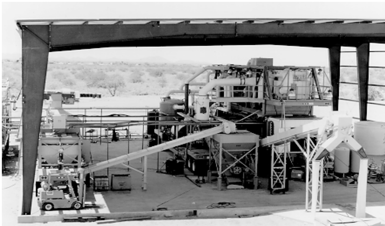
Desorption and Vapor Extraction System (DAVES)
