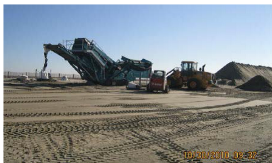
Figure 4.6-12. Top photo: “Big Dig” sifting operations on Pensacola Beach, Florida, on December 17, 2010. Bottom photo: “Power Screen Chieftain” sifting piles of oiled sand removed by mechanical scraping on Grand Terre II on October 30, 2010.
