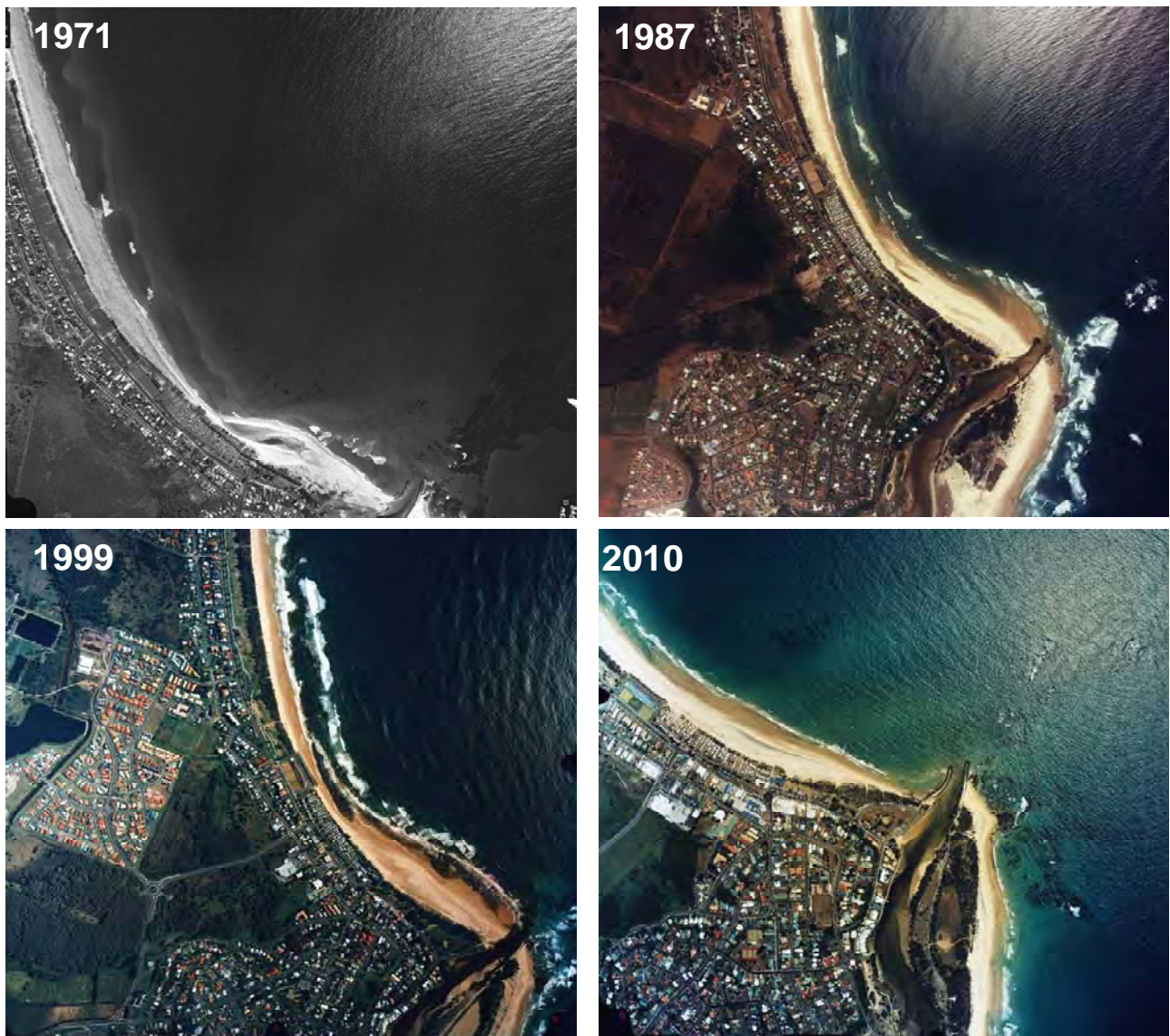
Figure 14 – Previous sand wave events that have occurred at Kingscliff. Three prior events on photographic record show the impacts of sand waves in 1971, 1987 and 1999 with erosion occurring along Kingscliff beach in front of the wave. The 2010 photo shows the beach state prior to the most recent 2011 sand wave, with sand shown to be building up on the southern side of Cudgen Headland, before its subsequent movement into the embayment.
