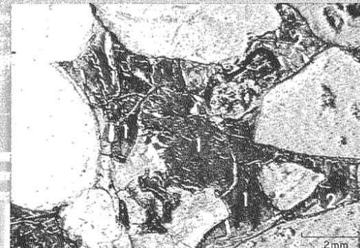
**j.** Secondary porosity (1) in leached plagioclase grain (2). Kaolinite clay (3) in a leached pore space. Frio Formation, Phillips No. 1 Houston "JJ" (15,829 feet), Brazoria County, Texas.
