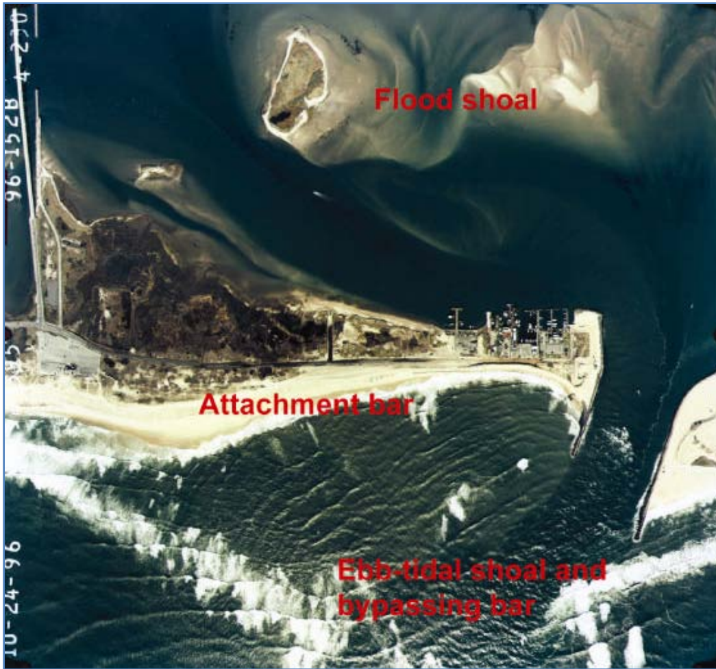
Figure 11. Shinnecock Inlet, Long Island, NY, illustrating the major morphological elements of the inlet.
