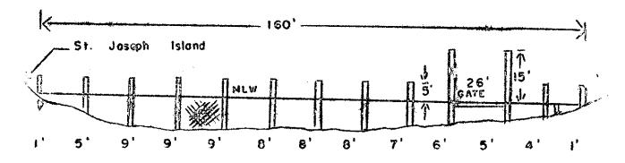
Side view diagram of proposed fish trap looking NE and showing nets and piling.
