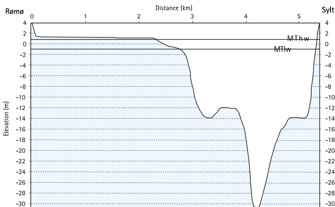
Figure 5.2. Cross-sectional diagram of "Lister Tief" tidal inlet.
