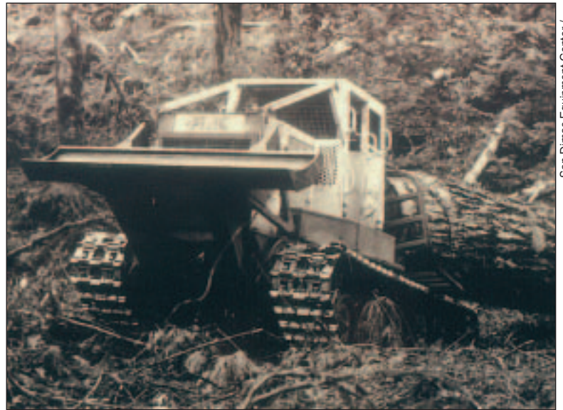
▲ Track vehicles with elevated pans also limit rutting.
