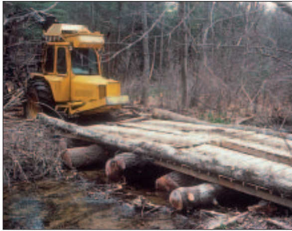
▲ These skidder ramps are lighter weight and will sometimes require logs for support.
