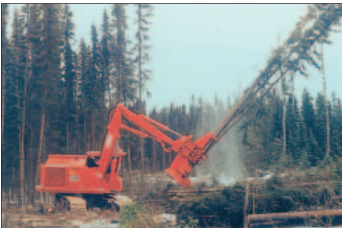
▲ This track vehicle fells and bunches trees, reducing the density of the skid trail pattern.
