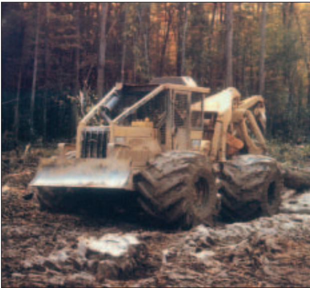
▲ High flotation equipment such as these extra wide tires helps to prevent rutting.
