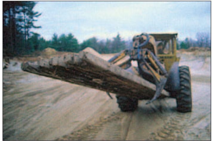
▲ The skidder bridge consists of two sections, permitting it to be carried and placed by the skidder that will use it.
