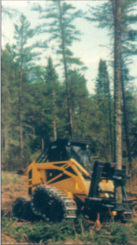
▲ This smaller feller/buncher uses a track system over rubber tires for versatility.
