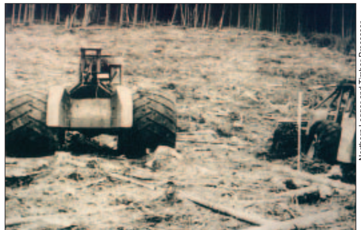
▲ Note the difference in rutting between wide tire (left) and conventional tires (right) in the same skidding situation.
